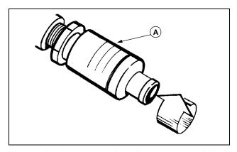
5. Unsnap the dust cap, push and twist to open oil drain (A) and drain oil into oil drain pan.
